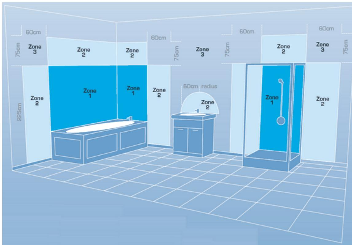
Bathrooms are considered to be a 'special location' for electrical installations because they have an increased risk of electric shock for the users, due to the proximity of water.
